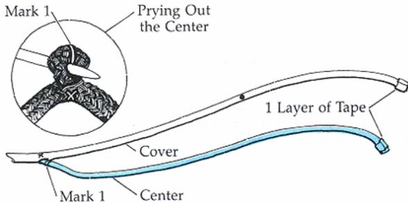
2. Pull out the core at **X** by bending the rope sharply and using the fid or a marlinespike to carefully pull out the core from in between the braids of the cover. Immediately mark the center core as **#1** with a single ring or unique color before pulling out the remaining core from **X** to the end. Tape the end of the core to keep from unraveling. If rope has paper tape inside the cover, remove all the way back to the slip knot.
