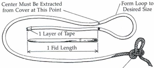
Tie a Slip Knot about 5 Fid Lengths from Point x
