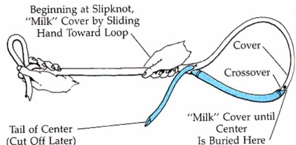
8. From the slipknot, "milk" the cover towards the eye and over the exposed center core. Gloves may be helpful to protect your hands when "milking" the cover. Continue until all of the center core and crossover are buried. Trim core tail and fuse.
