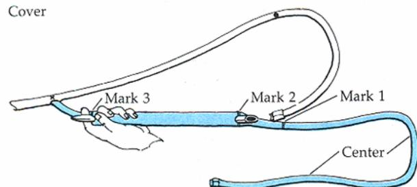
4. Insert the fid between the braids into the center core at **#2** and slide it through the "tunnel" until the point comes out at **#3**.
