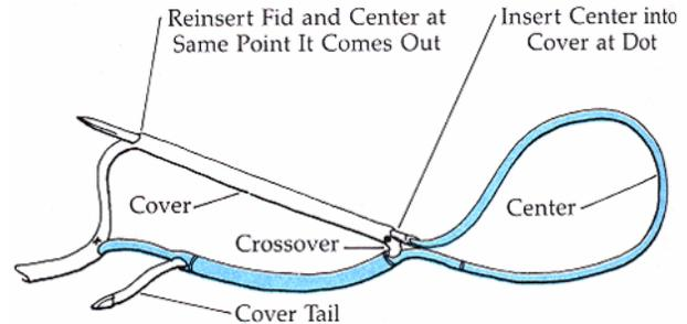
6. Now push the center core through the cover beginning at the **dot** and coming out at **X** using the same technique as in Step 5. Pull the center core through the cover until taugth then pull the cover tail at **#3** until taugth. With large eyes, multiple passes may be needed – simply re-insert fid at the point where it came out.
