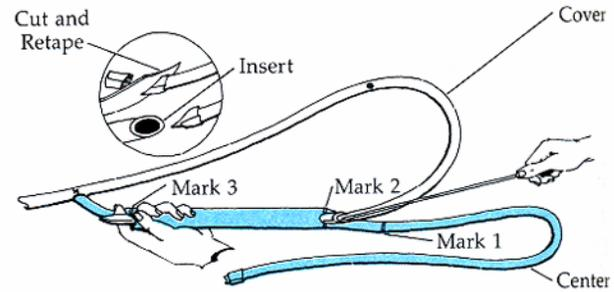
5. Cut diagonally across the tip of the cover to make a point and re-tape. If the final loop is to hold a shackle or other object, insert now. Jam this pointed end of the cover into the hollow end of the fid then use jam the pusher into the end of the fid securely and push the fid and cover through the center core until the **dot** on the cover almost disappears at **#2**.
