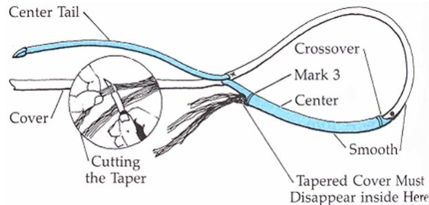
7. Unravel the cover tail braid all the way back to **#3** and trim the strands at different lengths to form a taper. Hold the splice at the crossover **dot** and smooth the center core until it covers the tapered threads of the cover tail and disappears into **#3**,
