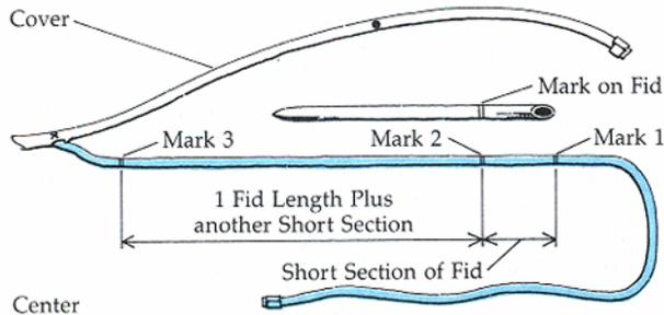
3. Pull out more of the center core. From mark **#1** measure a distance of one **short-fid** and mark **#2** as two rings or another distinctive color. Then measure a distance of one **short-fid plus one-fid** and mark **#3** as three rings or another distinctive color.
